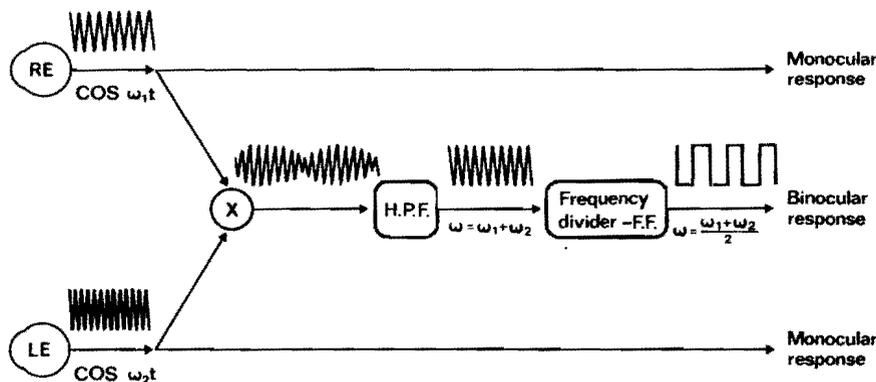
Fig. 1. Schematic diagram of a model of the visual system producing an intermediate frequency in binocular VEP. Under fusional conditions the multiplied signals from both eyes are shaped by the high-pass filter (HPF) and the frequency divider (F.F., Flip Flop). The output signal is a square wave of constant amplitude at the intermediate frequency.
